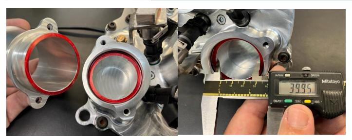
Issued restrictors are to be sandwiched between the throttle body and velocity stack mating surfaces, in direct contact with both surfaces. Those surfaces are colored RED in the images above. Note there is <u>not</u> a restrictor in these images.
