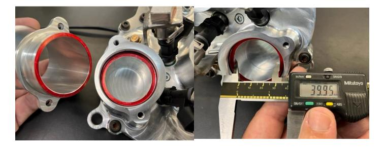
The throttle body inlet, where the issued restrictor contacts the throttle body, must maintain a continual circular internal dimension of 39.95mm +/- 0.1mm.
