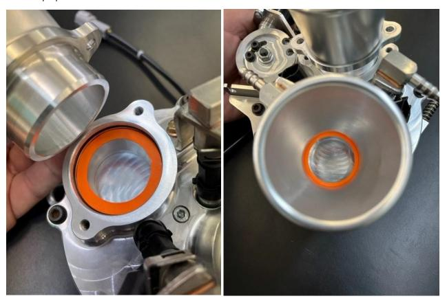
The velocity stack must have a continual circular chokepoint of 40.00mm +/- 0.1mm located within the length of the body. At no point within the entire length of the velocity stack can the I.D. be smaller than 40mm (same as 2023). *Supplementary* stacks cannot be inserted into or above the primary stacks to circumvent this regulation. AMA Pro Racing will make final determination of velocity stack compliance.
