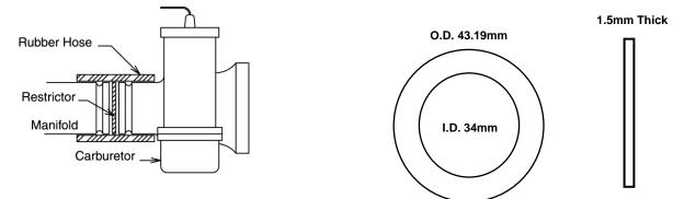
Issued restrictor dimensions: O.D. 43.19mm, I.D. 34mm, 1.5mm thick. Tolerance of +/- 0.15mm.
