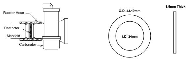
Issued restrictor dimensions: O.D. 43.19mm, I.D. 34mm, 1.5mm thick. Tolerance of +/- 0.15mm.
