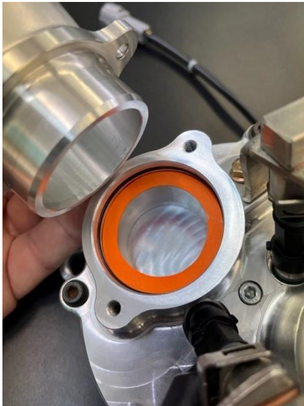
Restrictor location (left) and “down the stack” orientation (right). Orange “restrictor” shown for illustration purposes only.
