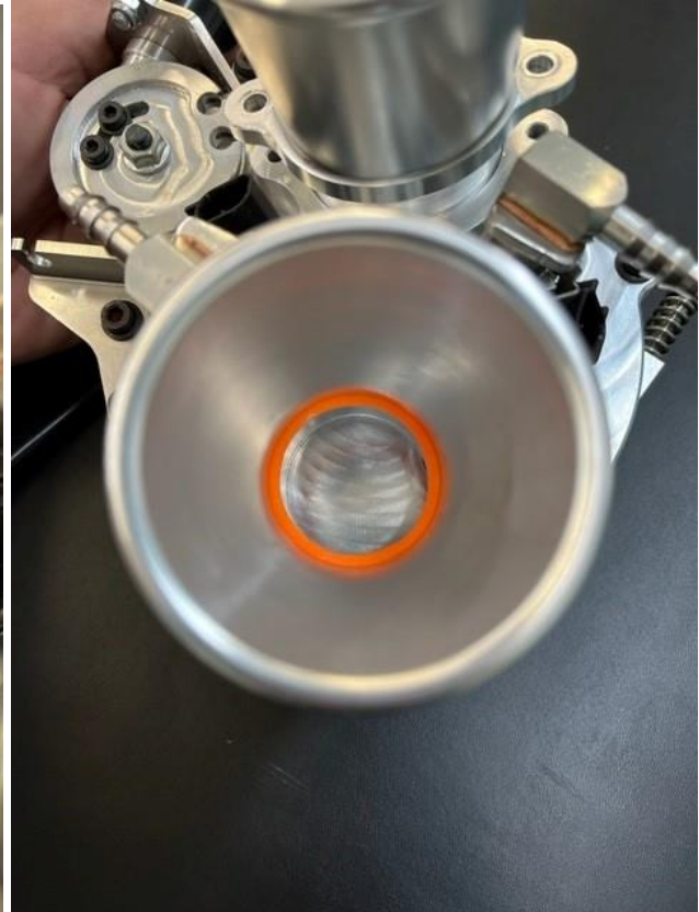
Restrictor location (left) and “down the stack” orientation (right). Orange “restrictor” shown for illustration purposes only.
